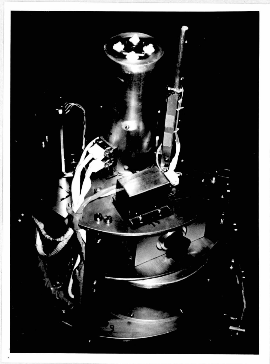
Figure 4.14 Close-up view of the mass spectrometer sensor on the rocket.
