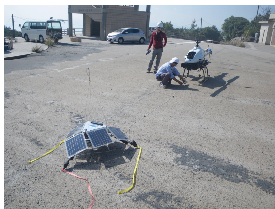
Photo 1 An unmanned autonomous helicopter and a seismic instrument with a solar power unit.
