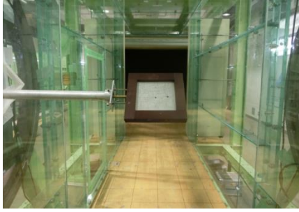
Fig. 4 Setup of aerodynamic force coefficient measurements.
