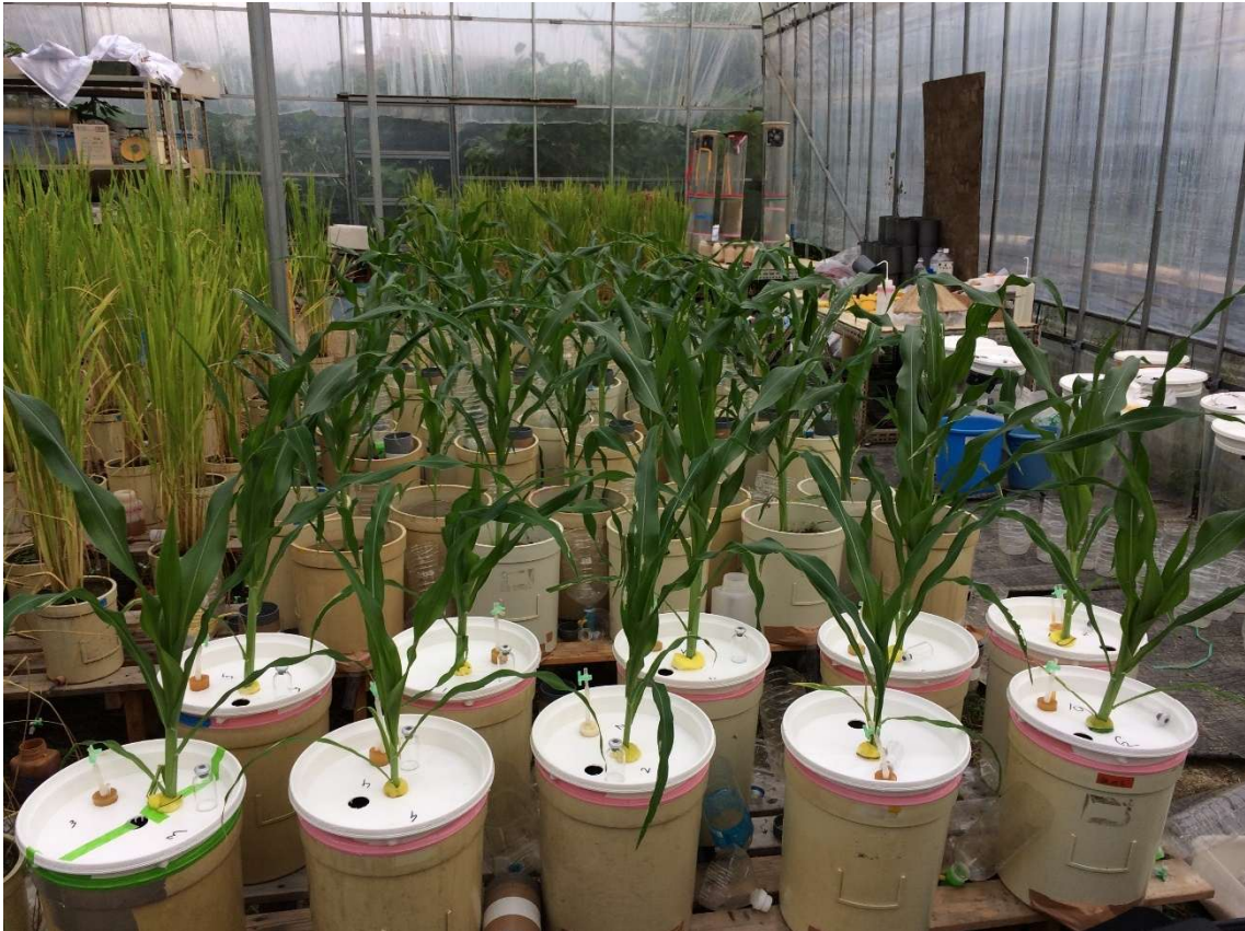
Picture 3: The modification of gas collection for maize in the first season
