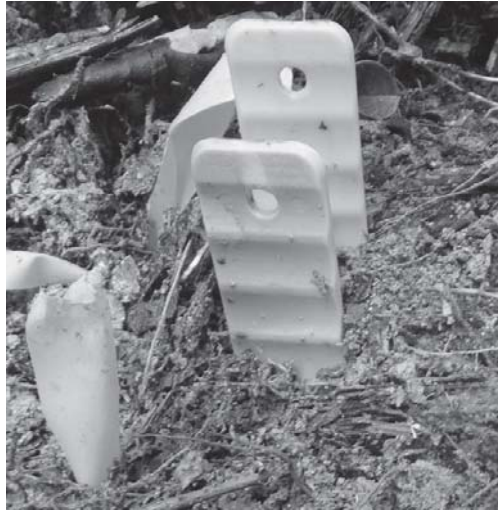
Fig. 1 The Plant Root Simulator (PRS) probes buried in soil for 2 months.
