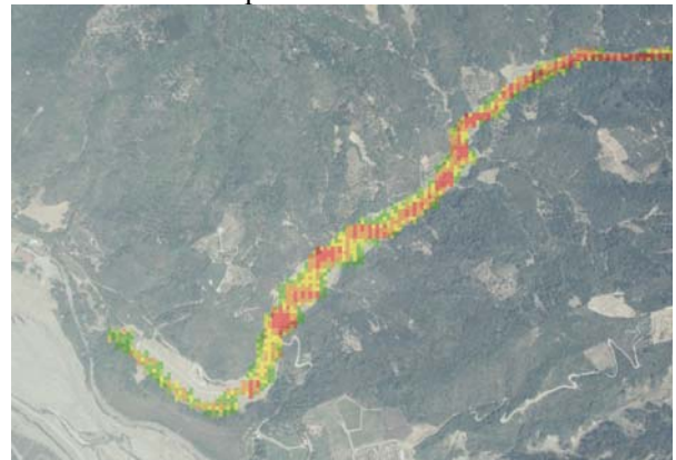
Fig.13 The simulation result – Nantou072, the depth in levee case
