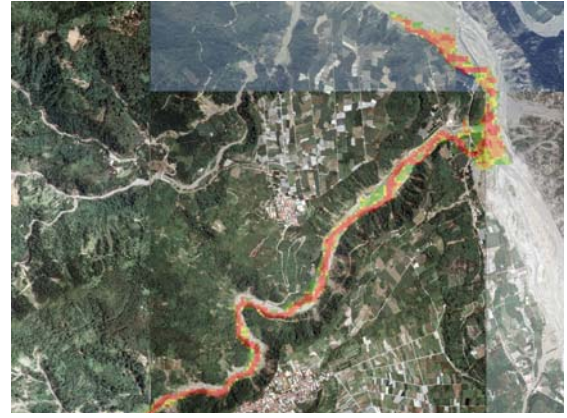
Fig.12 The simulation result – Nantou073, the depth in levee case
