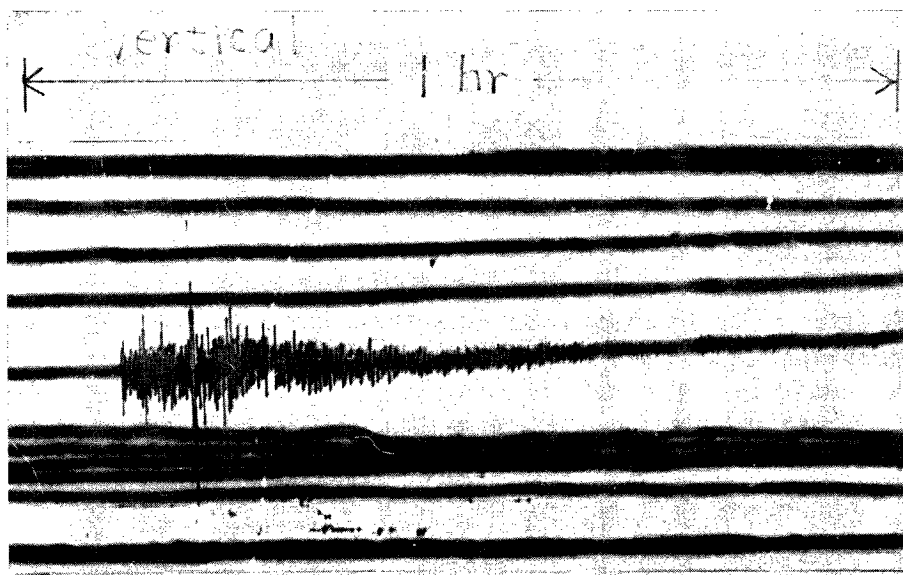
Photo. 1-(a) Photographic record of the vertical component of the strain seismograph at Ōtsu in the earthquake of Celebes Sea (June 12 th 01 hr. 45 m , 1972).
