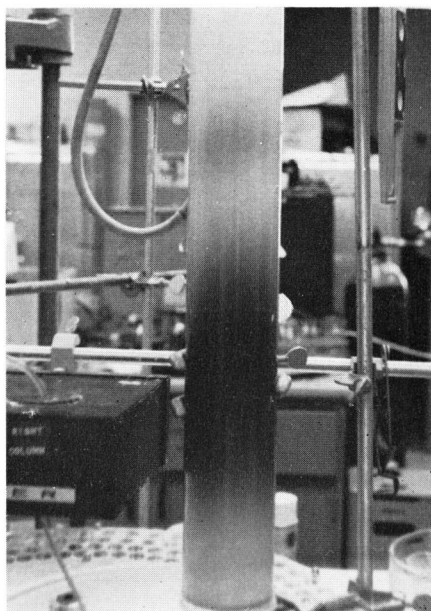
Fig. 20 Separation of myoglobin (the upper band) and hemoglobin (the lower band) with Sephadex G-75 column chromatography (0.005M NaCl).
