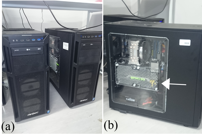
Figure 2.3 My GPGPU machines equipped with NVIDIA GeForce GTX TITAN and Tesla C2070. (a) A full view of the machines. (b) A side view. The graphic board is equipped at a position indicated by the arrow.
