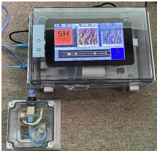
Photo 1 : Prototype of a simple seismic intensity meter. The upper side of the photo is the main unit including Raspberry Pi, and the lower side is the sensor unit including ADXL355 MEMS accelerometer. The dimensions of the main unit is 19cm x 28cm x 10cm, while that of sensor unit is 10cm x 10cm x 6cm.
