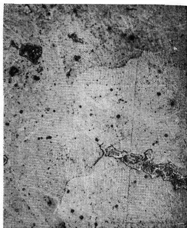
Photo. 1 \times 300 C=0.16%, As=3.31% 900°C. \times 2 hr. F.C. 5% Picral etch. Ferrite + Pearlite.
