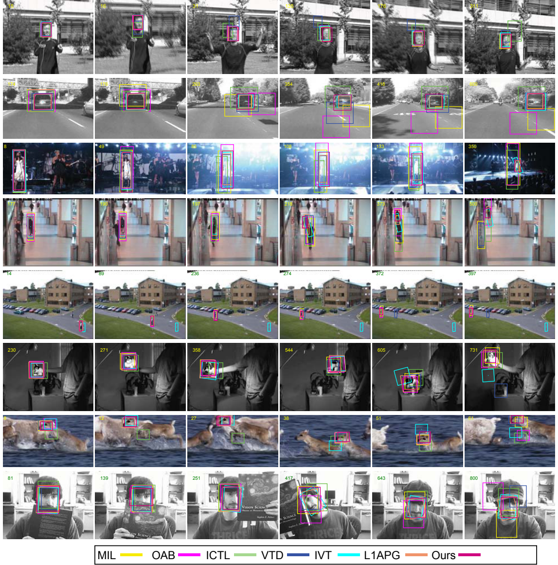
Figure 5.5: Tracking results of different algorithms for sequences Jump, Car4, Singer1, Walking1, Walking2, Sylvester, Deer, and FaceOcc2.
