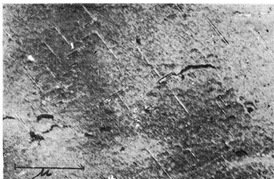
Fig. 3 Al-Cu Alloy aged 30 hr. at 200°C
