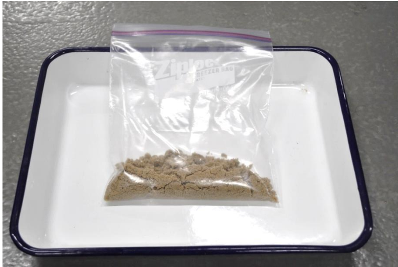
Photo 3.2 Mixture of Toyoura sand and water with a certain water content
