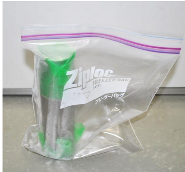
Photo 3.5 Mold packed in a plastic bag
