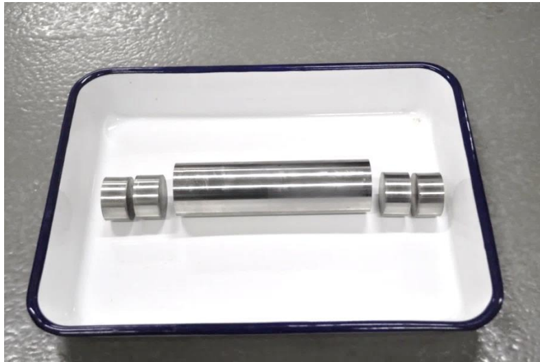
Photo 3.4 Mold for freezing the moist sand and spacer blocks
