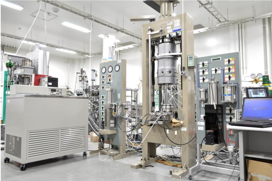
Photo 3.1 Exterior appearance of temperature-controlled high-pressure triaxial apparatus
