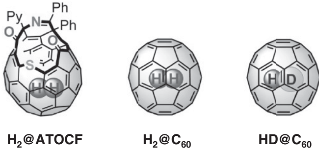
FIG. 1. The hydrogen endofullerenes H 2 @C 60 , HD@C 60 , and H 2 @ATOCF. (ATOCF: azacyclic-thiacyclic open-cage fullerene).
