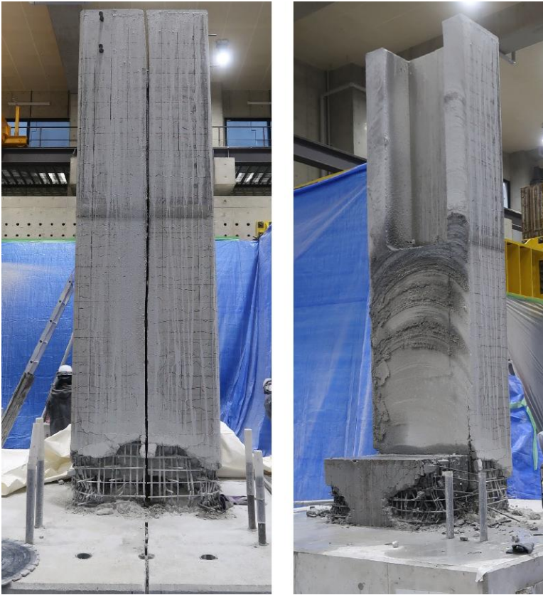
Fig. 9. Cutting at the center of the cross-section to examine internal damage.
