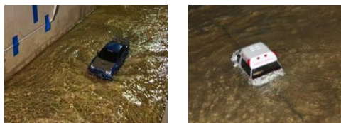
Photo 4 Floating model car in the experiment
