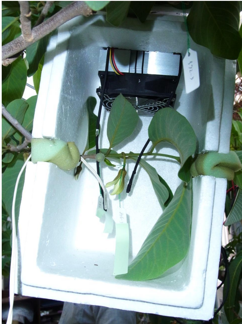
Fig. 3.3 A styrene foam box equipped with the temperature control device (Fig. 3.1), being installed on the tree to enwrap a cherimoya flower.
