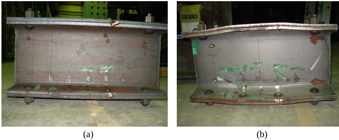
Figure 5.6 Residual deformation: (a) HT-120; (b) CT-120.
