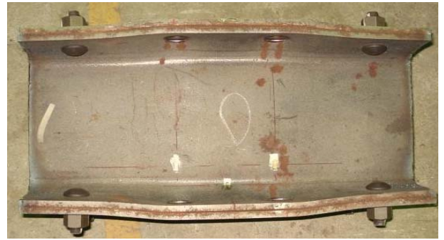
Figure 5.10 Comparison of residual deformation (CT-120): (a) a picture from the finite element analysis; (b) a photo from the test.
