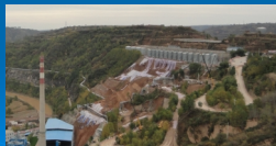
Yanlian landslide in Shaanxi Province triggered by water leaking
