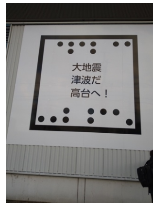
Photo 10 Example of AR marker
